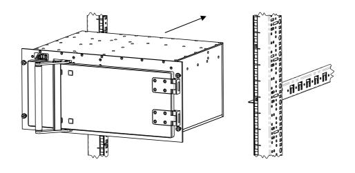
4 Mark the positions from the front plate to the breakouts in the L-profile. At this position the cage nuts (figure 4) have to be installed.
