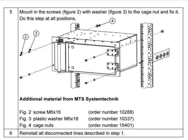
Table 1: Work steps for install the Shielding Boxes in a mounting device
